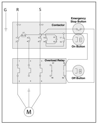
Figure 89. G0591 single phase wiring diagram.
